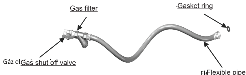
14. picture: Attachment with flexible pipe (option, it can be purchased at the appliance manufacturer)
