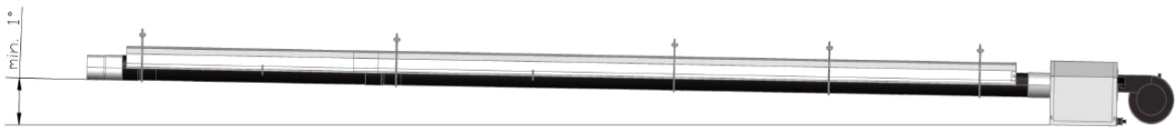
28.picture Minimal ascent of installation
