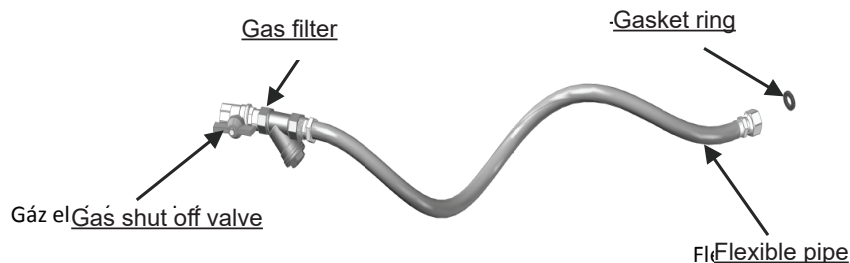
14. picture: Attachment with flexible pipe (option, it can be purchased at the appliance manufacturer)
