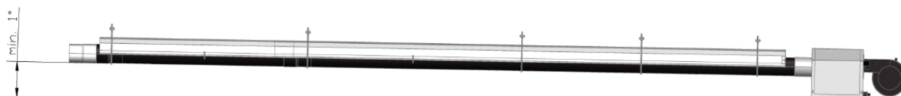
10. picture Minimal ascent of installation
